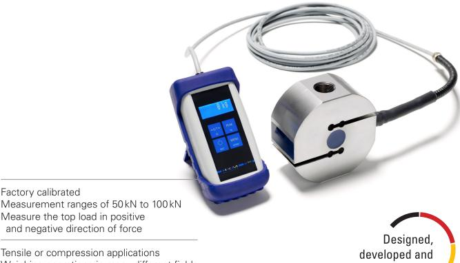
Measure the top load in positive and negative direction of force
