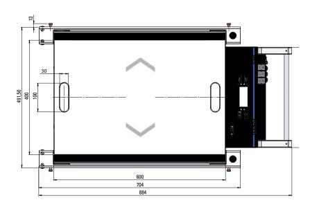
Weighing area L 400 mm x W 600 mm Height 45 mm
