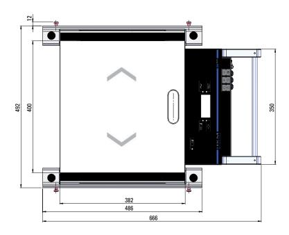
Weighing area L 400 mm x W 382 mm Height 40 mm
