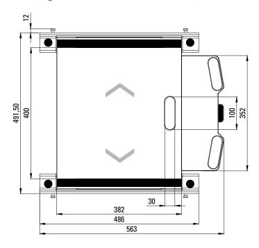
Weighing area L 400 mm  $\times$  W 382 mm Height 40 mm
